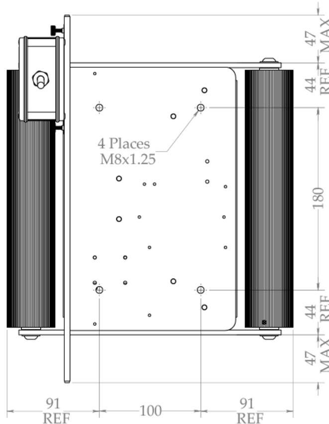
Fig. 6: Mounting hole pattern
