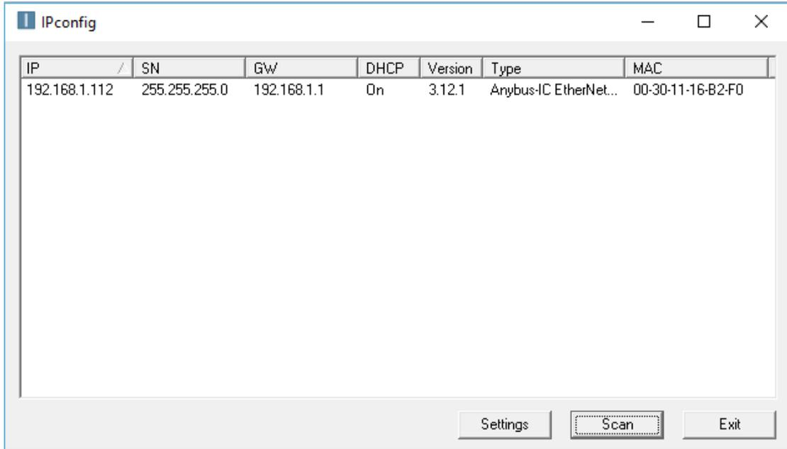
Information such as IP address, DHCP state, Type of module and the MAC address is displayed.
