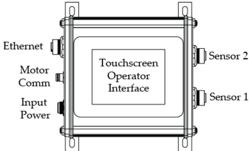
Fig. 10: ARIS SCU5 connector ports
