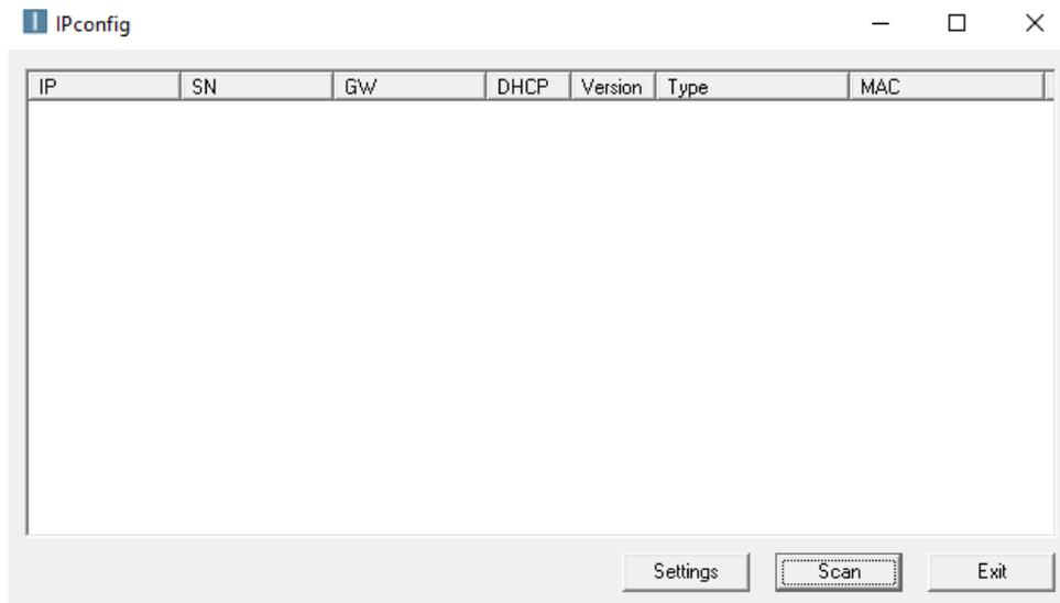
By pressing the scan button all the devices on the network from HMS Industrial network can be found. For example, the utility would find the device and list it as shown below.
