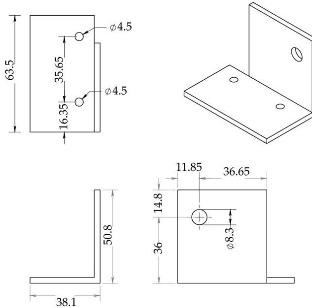
Fig. 15: Servo Center Sensor Mounting Bracket (All Dimensions in mm)
