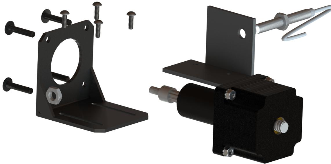
*Fig. 16: The Components of the Actuator and Servo Center Sensor Assembly*
