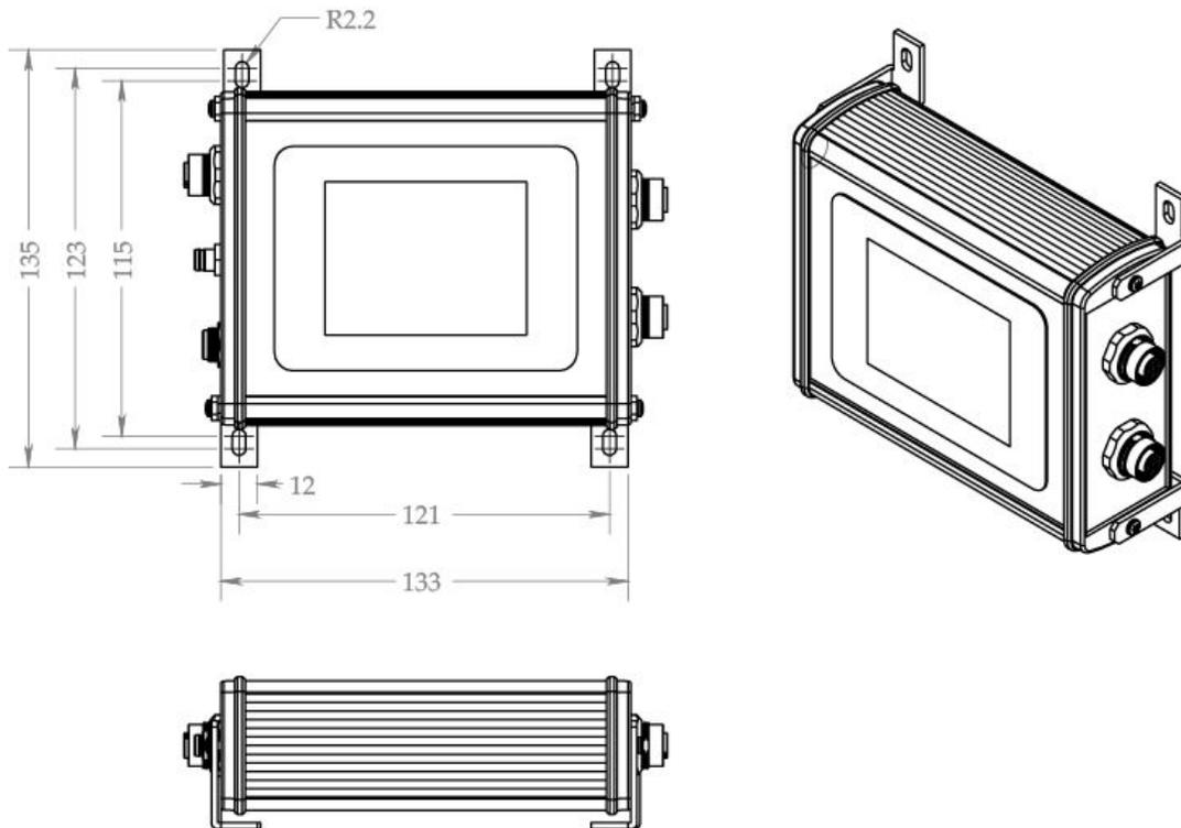
Fig. 10: SCU5 Controller Physical Dimensions (All dimensions are in mm); Subject to change without notice.
