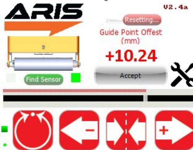
Fig. 24: Guide point reset
