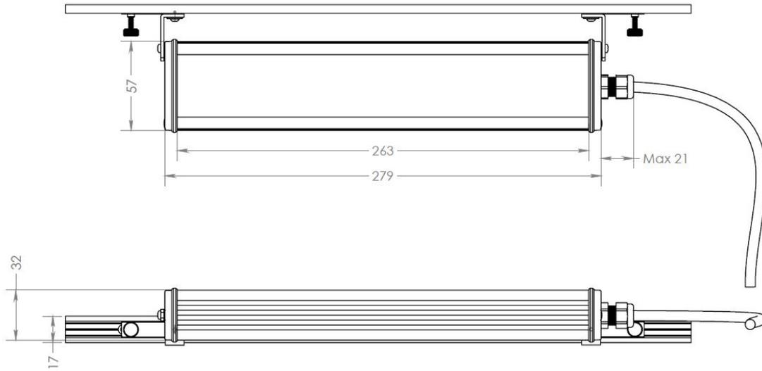
Fig.7: 221mm Sensor Head Assembly Dimensions (All Dimensions are in mm)
