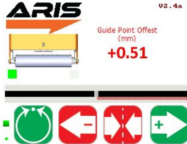
Fig. 22: Fine guide point adjustment
