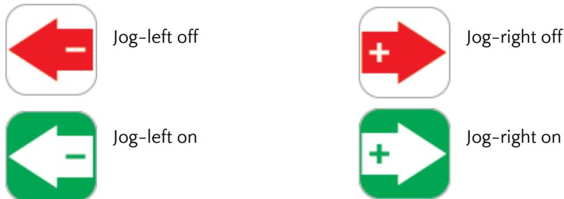
The Jog-left/Jog-right icons allow the operator to manually move the guide roller assembly to the left or to the right as needed. These operations can be performed only when the web guide is in manual operating mode.
