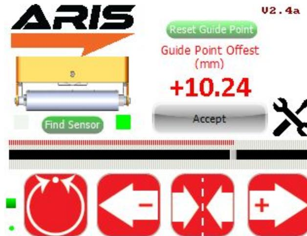
Fig. 23: Gross guide point adjustment
