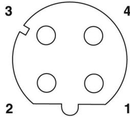
Fig.12: 4- Pin Industrial Ethernet Connector.
