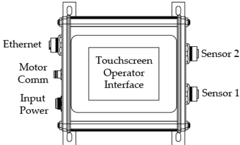
*Fig. 11: SCU5 Connector Ports*
