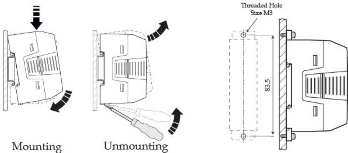
Fig. 18: DIN Rail and Wall Mounting Options
