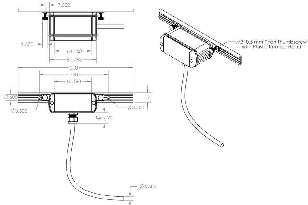
Fig. 6: 48mm Sensor Head Assembly Dimensions (All Dimensions are in mm)
