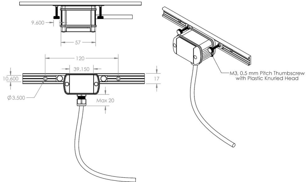
Fig. 5: 16mm Sensor Head Assembly Dimensions (All Dimensions are in mm)
