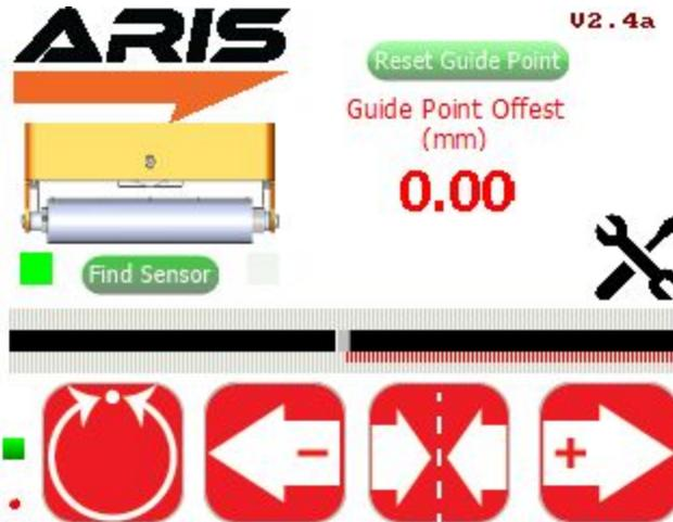
Fig.19: ARIS Operator Interface (Manual Mode)
