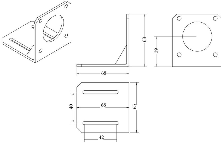
Fig. 14: Actuator Mounting Bracket (All Dimensions in mm)
