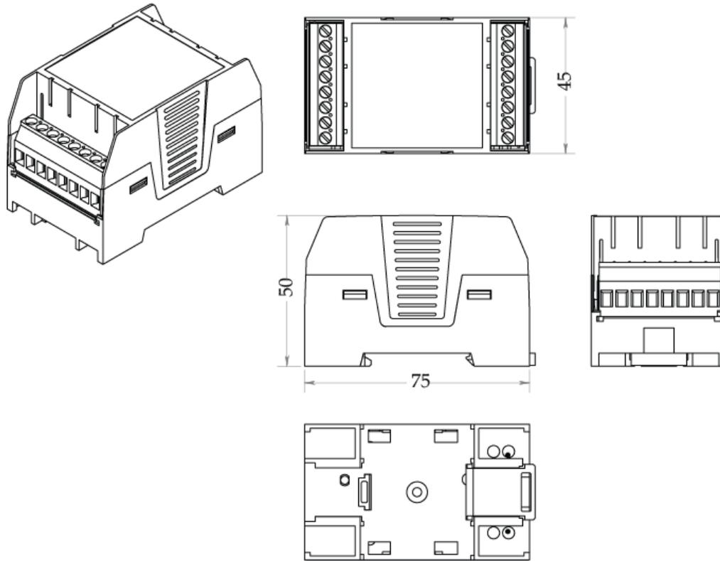
Fig. 18: Physical Dimensions of the Microstepping Driver (All dimensions in mm)
