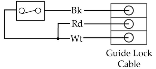
In case the case where there is no need for a guide lock switch, all the three conductors can be shorted to enable the web guide to operator normally all the time.
