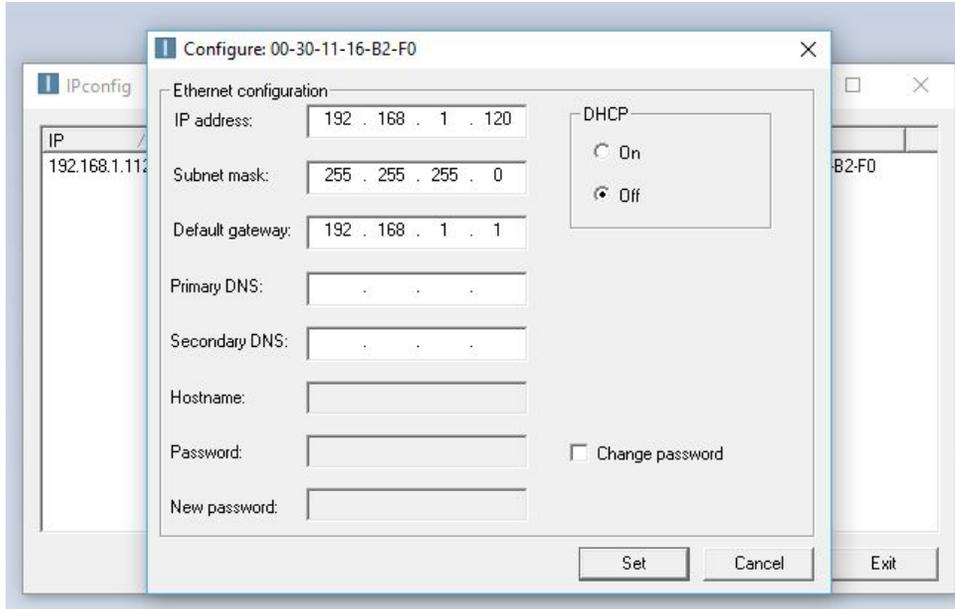
By clicking on the “Set” the static IP address can be set. Once the static IP address is set the IPconfig utility will refresh to show the new configuration. The DHCP setting will be set to “OFF” state and the new IP address will be assigned to the device as shown below.
