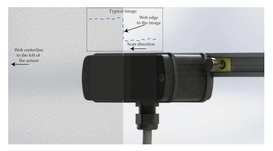
The digital web position or the edge position is the pixel number at which the edge transition is seen. The corresponding analog output is proportional to the percentage of the sensing window covered by the web. For example, if the digital edge position is at 256th pixel (with ARIS WPS 48), the analog output is 33.33% of the output range or 3.333 V for a sensor with 0 to 10 V output range.
