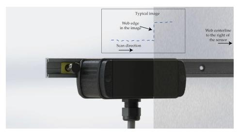
The analog output from the sensor will provide a signal proportional to the web edge position. Specifically the analog output is proportional to the portion of the image covered by the web. For example, with a left sensor orientation if the edge is located at the 569th pixels (with ARIS WPS 48), the analog output would be the percentage of sensor covered by the web multiplied by the output voltage range.
