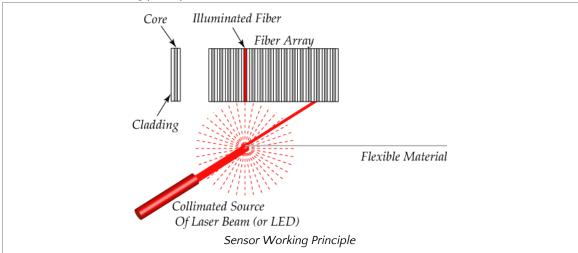
A schematic of the basic working principle is shown below:
