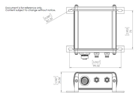
The driver can be mounted in a machine cabinet or on the machine frame close to the web guide, as long as the enclosure is properly grounded. The mounting screws or the wall mounting brackets can be used for grounding purposes.
