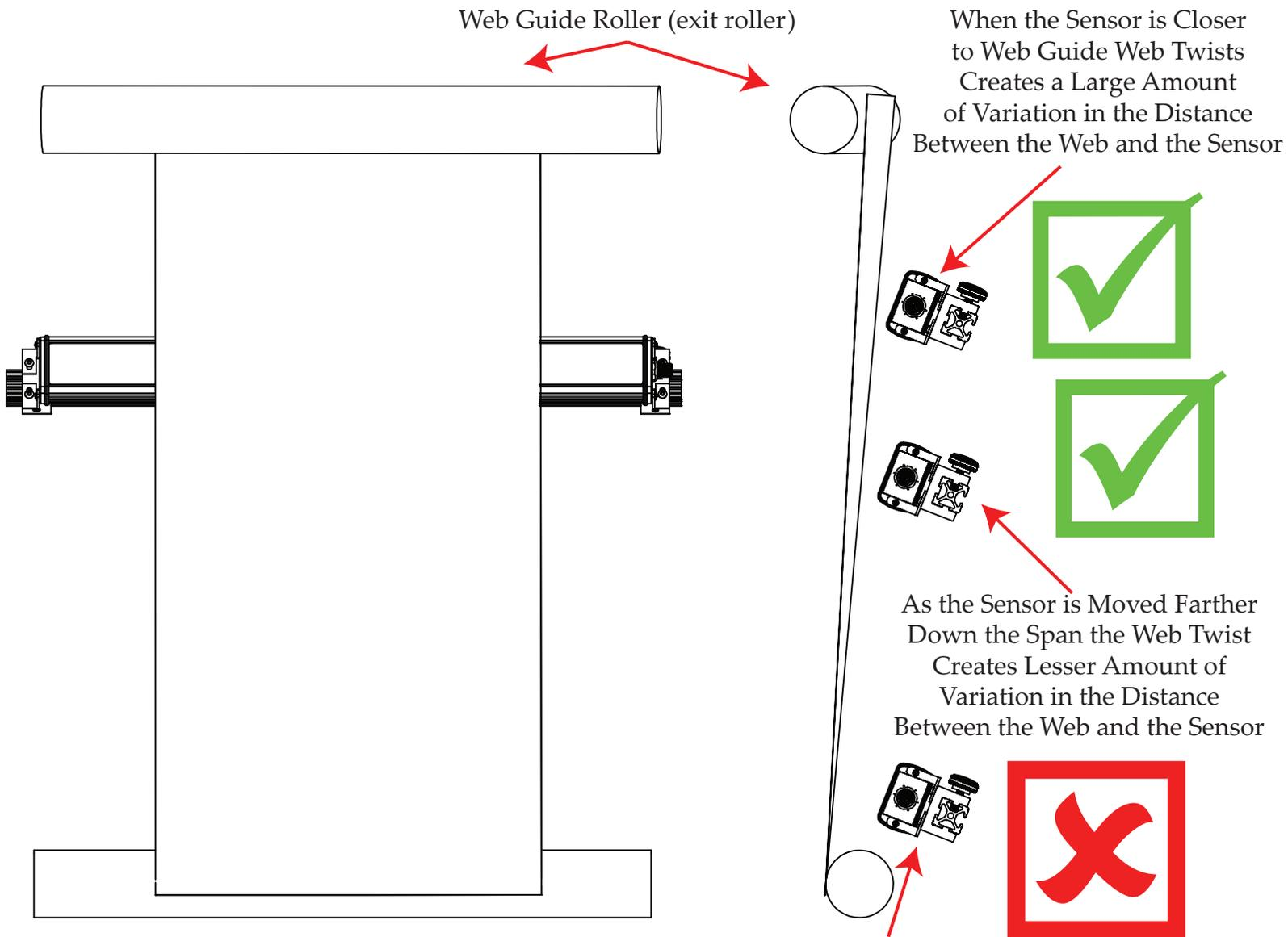
Even Though the Effect of Web Twist Will be Small in this Location it is not Recommended to Install the Sensor in the Second Half of the Exit Span
