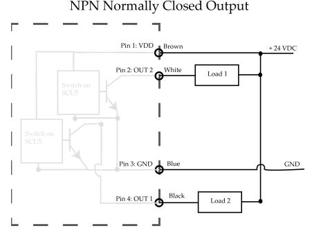
When the respective output signal is enabled then that signal would go low. And normally the signal would be high if wired as shown in the schematic on the left.
