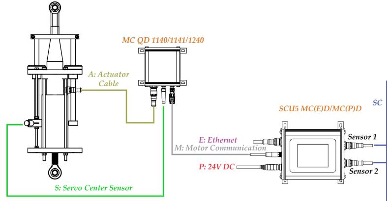
SC: Quick Disconnect Sensor Cable M12 12-pin shielded cable Male and Female cordset
