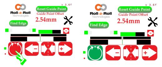
Step 7: If needed use the fine guide point adjustment to fine tune the desired web location.
