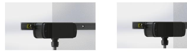
Step 5: On the SCU5 operator interface ensure that the two edges are seen by the controller and reset the guide point.
