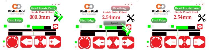
Step 6: Press the Automatic/manual button to put the web guide in Automatic Mode.
