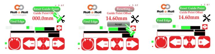
Step 6: Press the Automatic/manual button to put the web guide in Automatic Mode.Step 7: If needed use the fine guide point adjustment to fine tune the desired guided web location.Note: This procedure is for the right sensor mode but the same procedure is applicable for left sensor mode as well.
