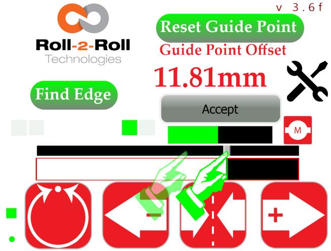
Figure 5.29: Release of track bar will prompt confirmation of the new guide point offset
