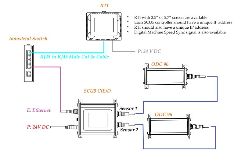
SC: Quick Disconnect Sensor Cable M12 12-pin shielded cable Male and Female cordset
