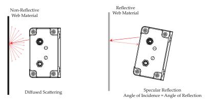
Figure 20: Diffused scattering with non-reflective webs and specular scattering of reflective webs may require different sensor rotation.
