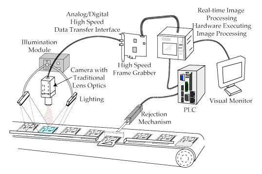
Figure 3: Complexities of Traditional Machine Vision Systems
