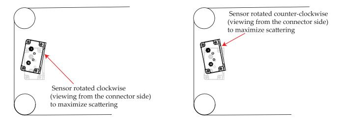
Figure 23: Sensor oriented to maximize scattering
