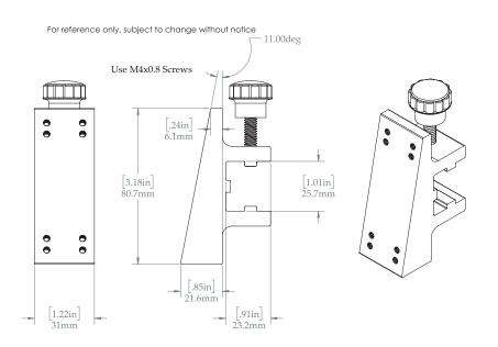
Figure 25: Angled 1" Sensor Mounting Bracket for use with 1" extrusion or 25 mm extrusion
