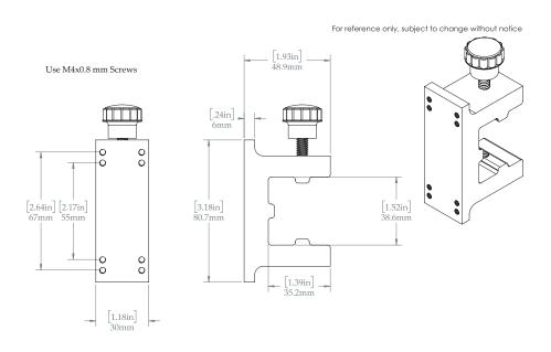
Figure 17: 1.5" Sensor Mounting Bracket for use with 1.5" extrusion
