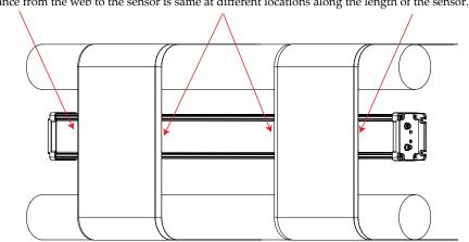
Distance from the web to the sensor is same at different locations along the length of the sensor.
