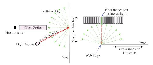
Figure 1: Scattering and Spatial Filtering Technology
