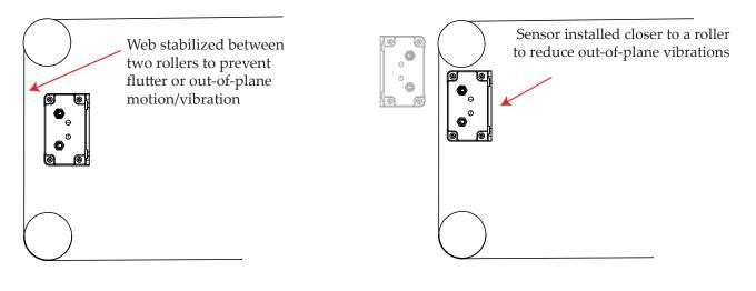
Figure 21: Sensor installed between two fixed roller for inspection applications
